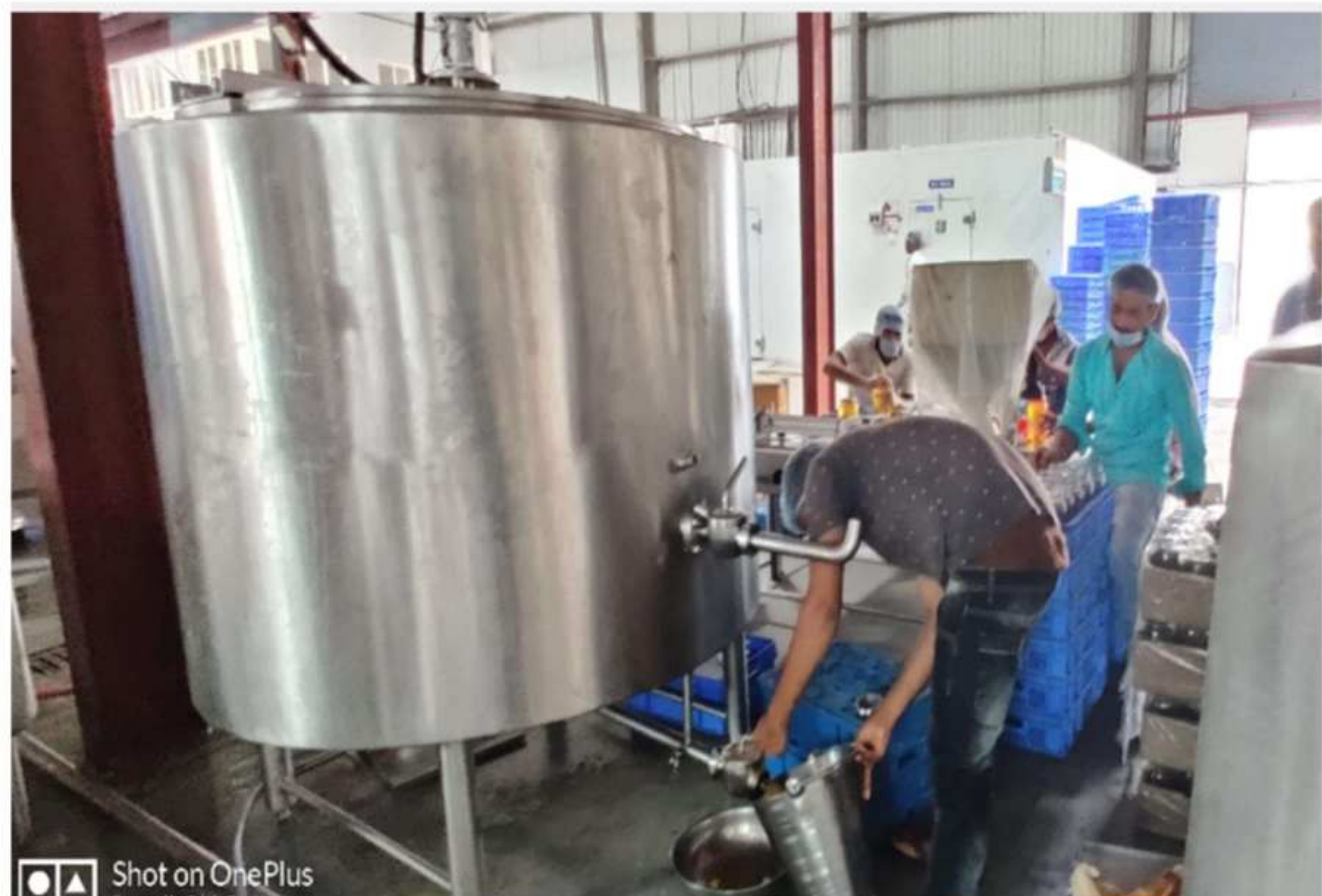
GHEE SETTLING TANK
