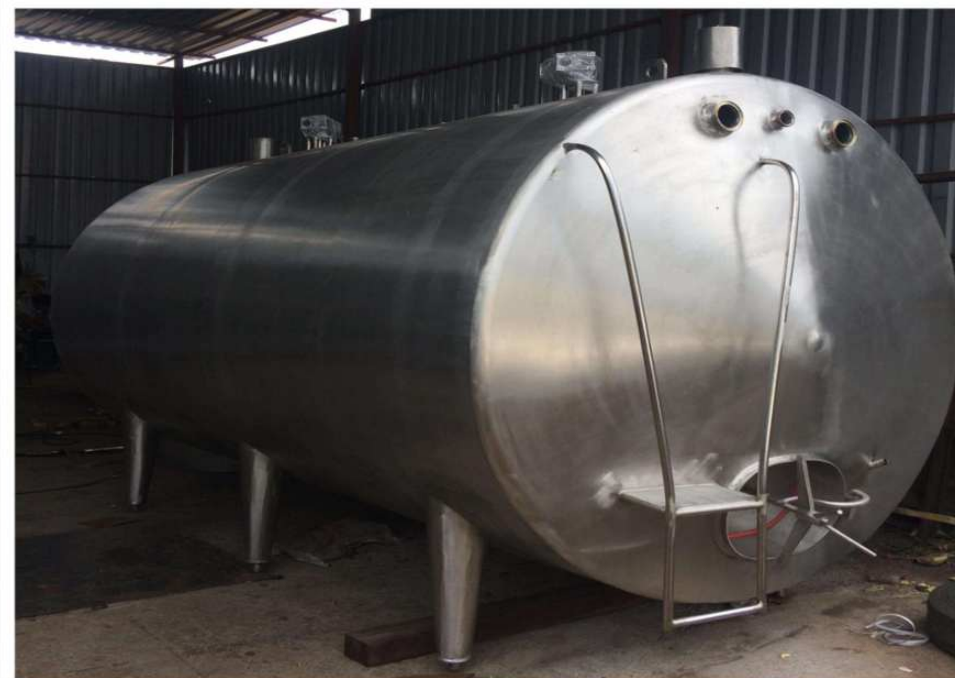
MILK STORAGE TANK
